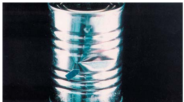
3 If the body dent does not significantly affect the side seam or double seams.
